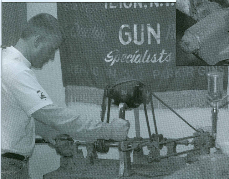
Lawrence Del Gego demonstrating safety slot drilling jig.
