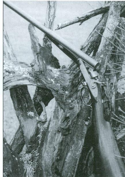
Bob Davis dollar grade Parker, showing the filed contour of the frame behind the breech, and the cross slide forend attachment.
