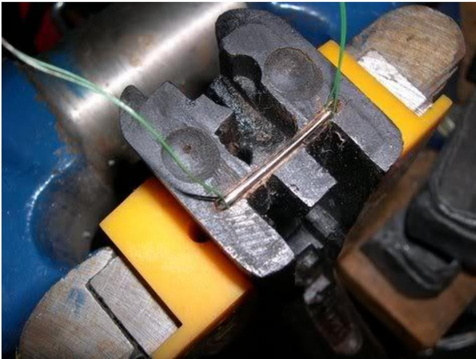
Finally, using a straight-edge to make sure that the crossbar of the staple is well-below flush with the face of the stockhead
