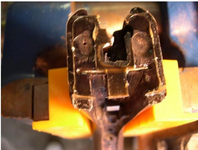
Another view showing the footprint of the receiver on the stock, outlined by the excess epoxy
