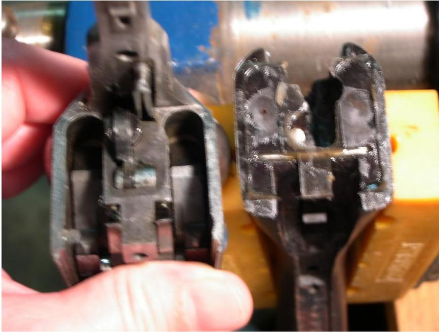
I just realized that one of my pics fortuitously illustrates the observation I made earlier about the original wood-to-metal contact being typically better around the edges of the stock than in the center, thereby concentrating recoil force around the outer surface.
