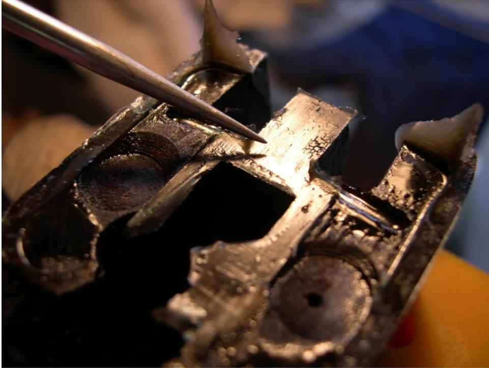
Don't forget to put release agent on the small part of the trigger plate that comes in contact with the wood when assembled (I have, but remembered before I tried to assemble it to the stock which had the epoxy already applied.) To forget could lead to a stuck triggerplate. Here's the release agent being removed from the mentioned area
