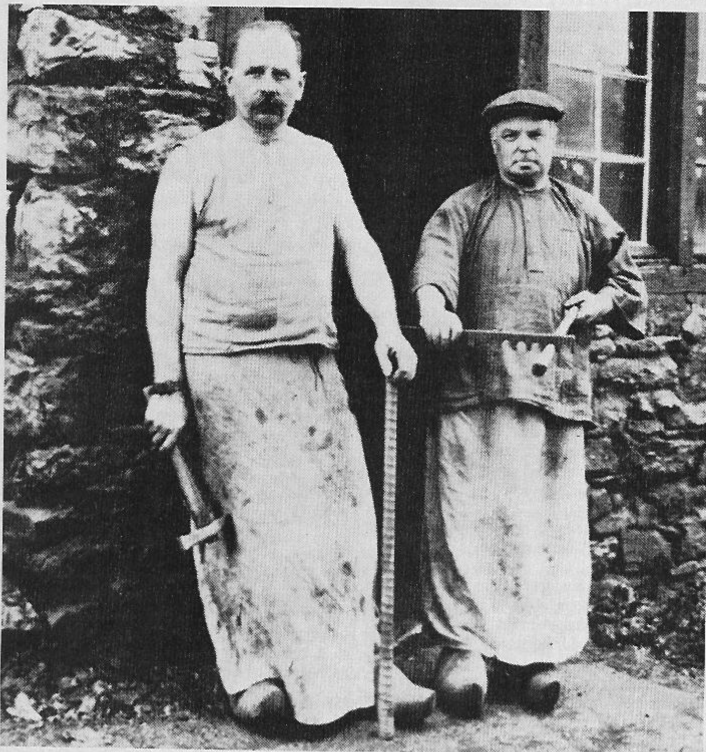
Barrelmakers outside their forge. Man at left is holding a roughed-out barrel; the one at right is checking the outside diameter of a hammered barrel using a gauge called a hanchon. (Plate 3)
